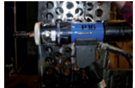
Internal bore welding (I.B.W.)
