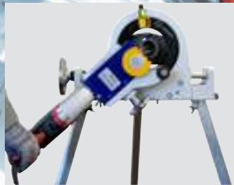
Cutting thin-walled stainless-steel tubes and elbows
