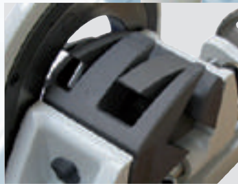
Deformation-free clamping of thin-walled tubes
