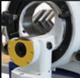
Second saw blade position to cut off elbows
