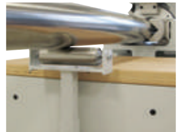
Roller pipe support
